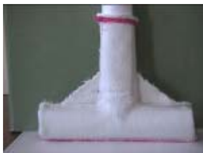
Fig. 3. T-tubular form with lateral reinforcement produced with glass fibre
