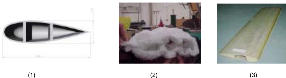
Fig. 10. Application of a sandwich structure for aeroplane wing (1) Wing section (2) Knitted preform (3) Composite
